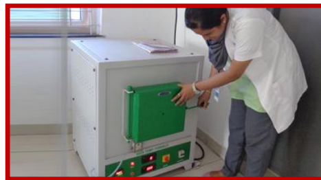
Precision Techno high temperature Muffle furnace : Used for solvent removal, sterilizing, evaporation, polymer curing, polyimide baking, testing the sample at high temperature and to determine the percent of ash content in the synthesized material
