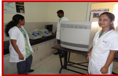
ABI 9700 HT fast real time PCR for SNP detection and DNA analysis
