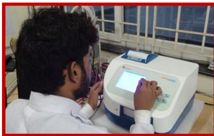
Elisa: Robonik Readwell TouchTM automatic ELISA plate analyser for routine immunoassays, biochemicals, hormones and drug levels can be carried out as it's versatile and extensive software support.
